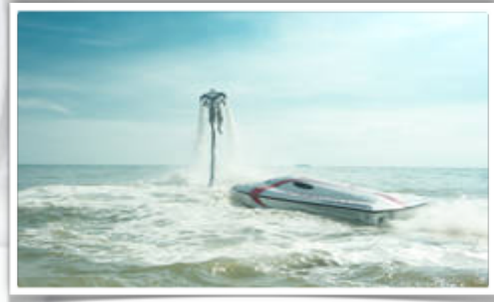
Above, the manufacturer of Jetlevs™ shows its Water Jet Devices (WJD—shown to the left) connected to a Personal Water Craft (PWC—at the right) by a high-pressure hose. Depending on the type of WJD, the PWC may or may not have an operator on-board.
